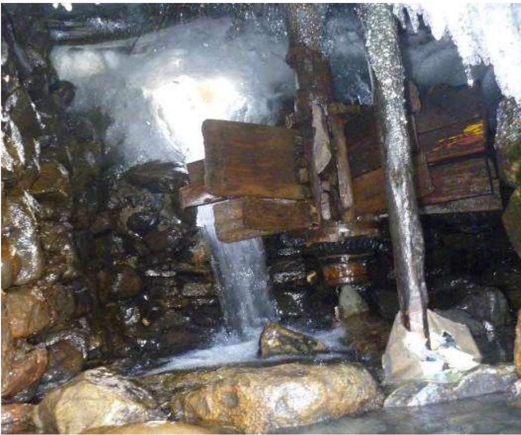
Left, the stream of water has been slowed (falling, lower center of photo) so Child Haven Manager Norbula could take Intern Robin Cappuccino into the basement of the barley mill. Full-force water turns the paddle wheel, which turns one of two stones above.
